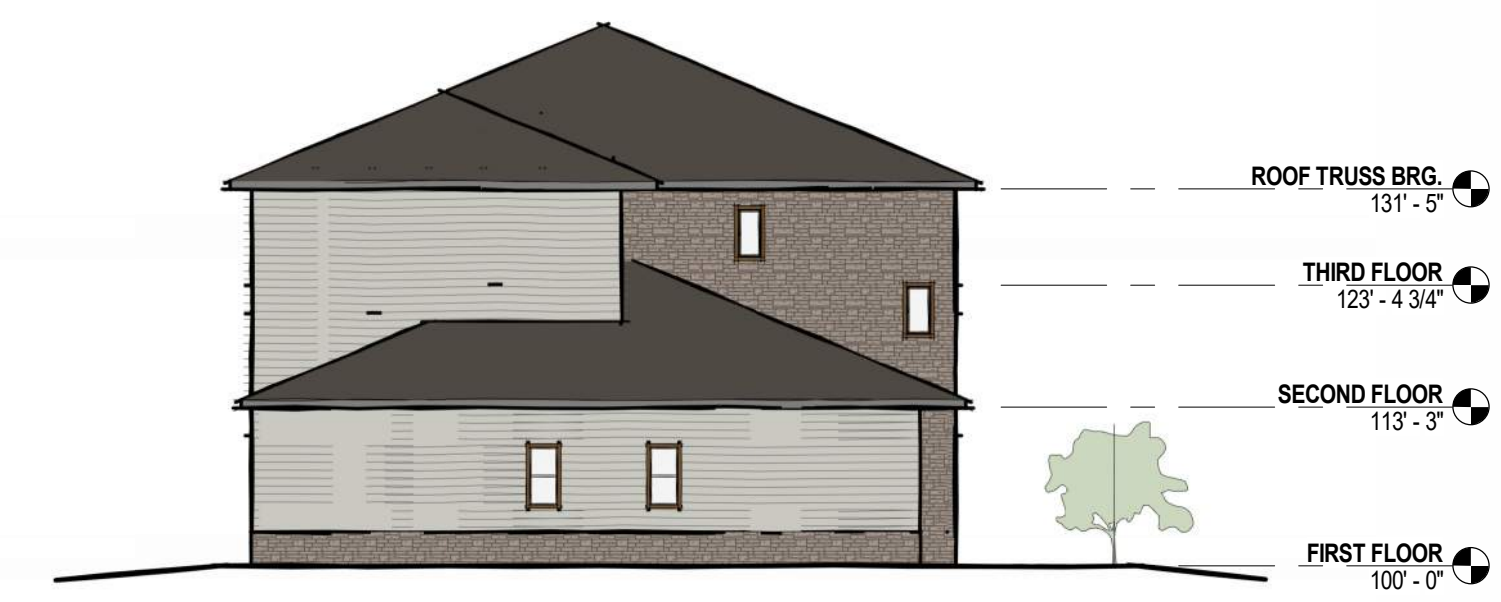
3 BUILDING ELEVATION - WEST 1/16" = 1'-0"
